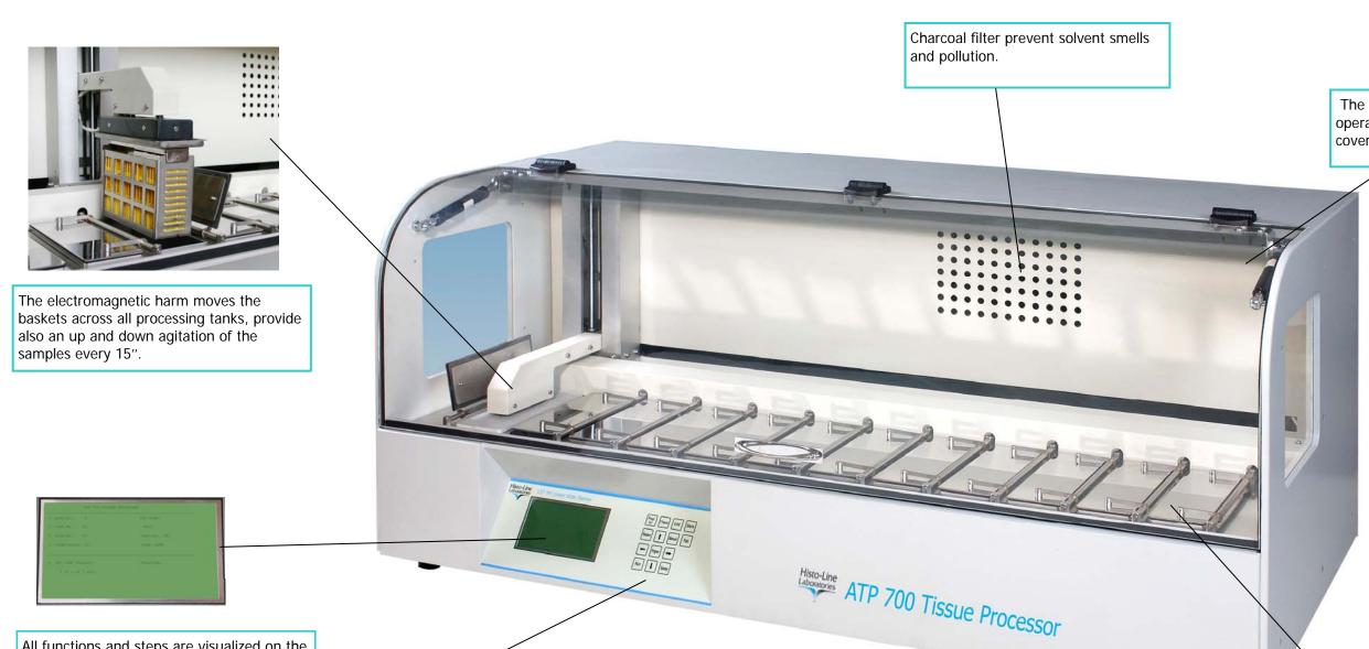
The environmental protection and safety of the operator is guaranteed by a plexiglass hermetic cover
